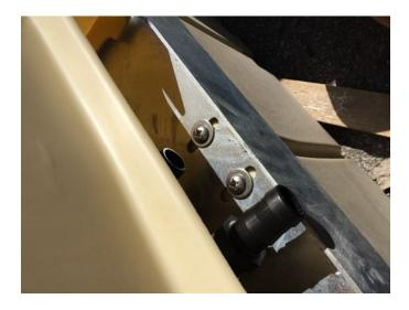
4. Slide supplied hose onto the fitting shown in the picture below, then tighten a hose clamp to secure the hose. Attach the other end to the float tank on the boat port, also with a hose clamp. The other fitting does not require a hose to be attached to it, as this is an air outlet vented to the atmosphere.
