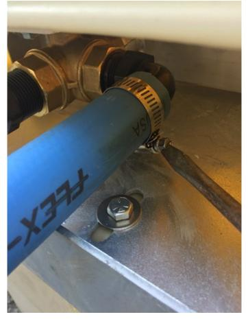
5. If you have purchased a 600052 or 600053 110V pump units, you may now plug the 110V plug to the 110V outlet. At this point, you can check to make sure the pump is operating normally via the remote option on the 600052 or the manual method on the 600053 pump. **NOTE: IT IS NOT RECOMMEND-ED TO RAISE THE LIFT TO THE COMPLETE UP POSITION WITHOUT A WATERCRAFT ON THE PORT.**
