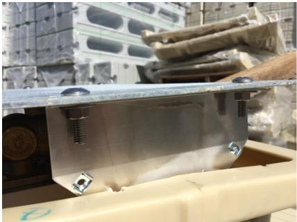
3. Next will be to bolt the bracket to the molded in t-nuts on the dock section using the 5/16 bolts and washers.
